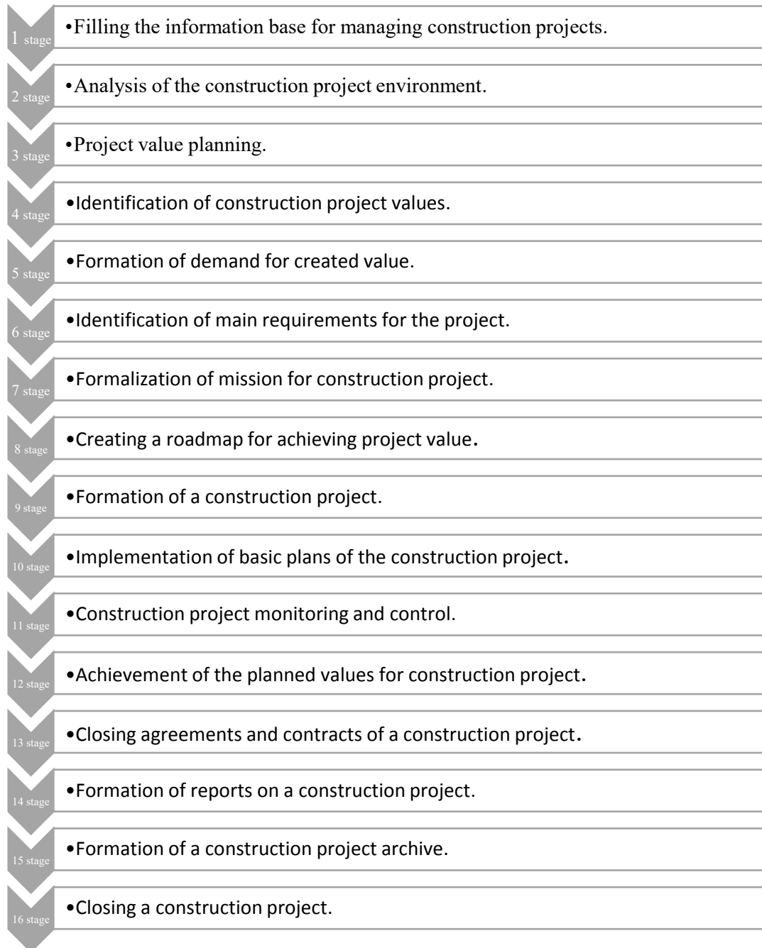
Fig 3. Stages of the method for determining the integrated value of a construction project
